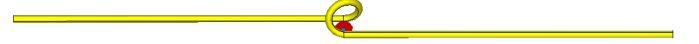
Fig. 1: Model of a wire-based harmonic tag with an inductive loop. A diode is attached in the air gap between the dipole arms.
