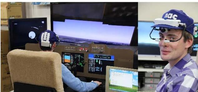
Fig. 4. The flight simulator and the NAC EMR-8 eye mark recorder. On the monitor on the left, a thresholded image of the subject's pupil is visible.
