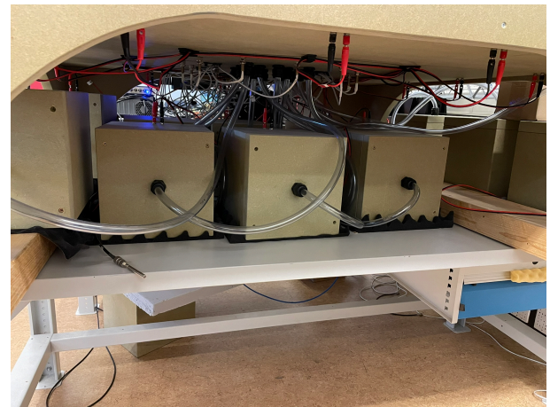
(b) The primary sources connected to the bottom of the experimental setup using tubes.
