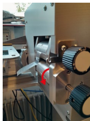
Figure 4: Labormaster HCT 3000 with the arrow indicating how the machine peels
