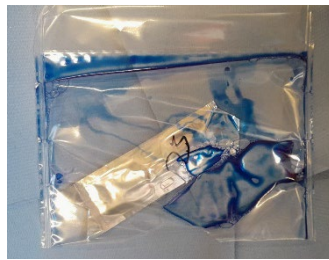
Figure 5: Dye penetration test with settings 0,1bar and 70%
