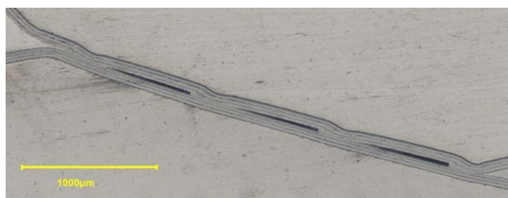
Figure 8: Cross section of an ultrasonic seal with four indents (OPE / PE-EVOH-PE (25/50) including controlled delamination easy peel with sealing settings 100% and 0,1bar)
