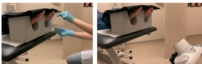
Figure 1.—Positioning of the feet of a healthy subject and of the portable HyperView™ camera at a standardized distance of 15 inches and perpendicular to the plantar side of the feet.
