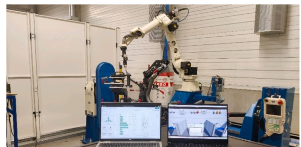
Fig. 7. The welding robot and representations of its digital twin [2].
