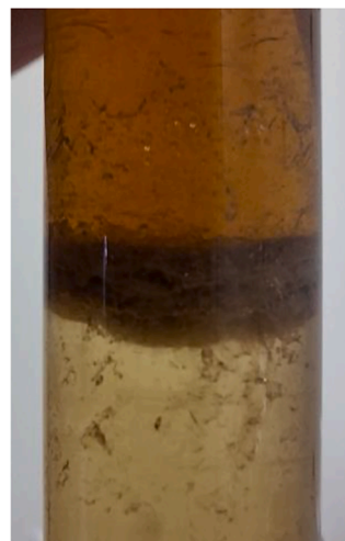
Fig. 16. Photo of centrifuge vial (10 mL total volume) containing ABH (top), Dowtherm A (bottom) and the solid phase that appeared on the interface.
