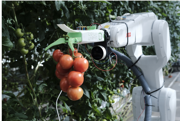
Fig. 4: The second generation gripper successfully manipulating a total of 11 tomatoes.
