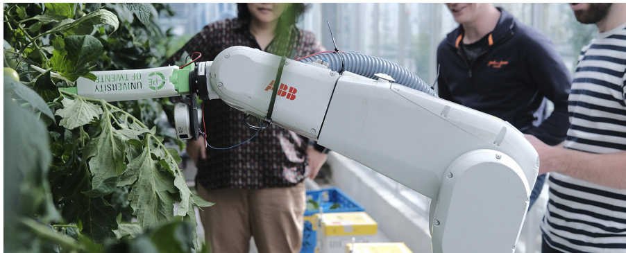
Fig. 1: The gripper attempting to grasp a tomatoe truss in a greenhouse environment.
