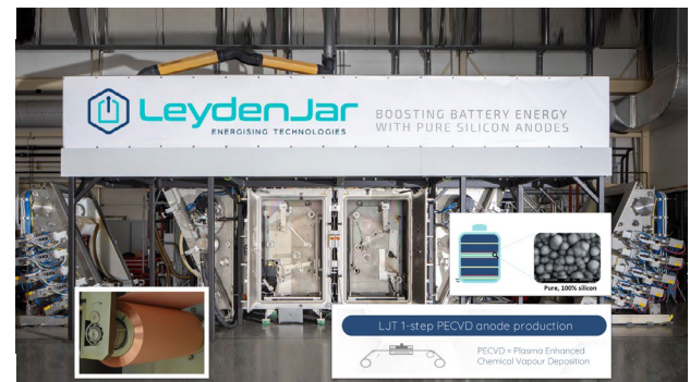
Fig. 6. One-step PECVD anode production machine in Leydenjar.
