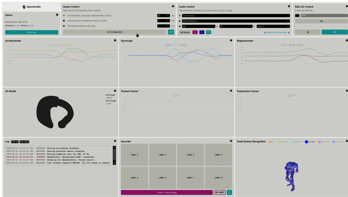
Figure 4: Augmented OpenEarable Dashboard, showcasing the recognition of a left roll in the head gesture recognition module in the bottom right
