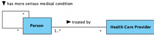
Fig. 3 A simple UML model describing a relation between Healthcare Providers and people treated by them.
