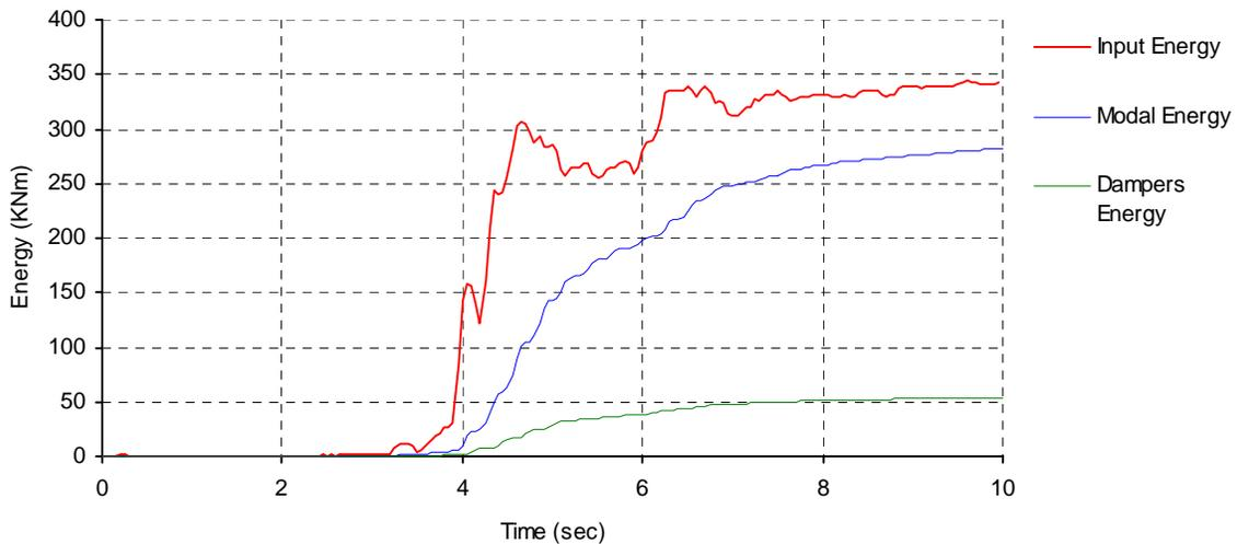
**Figure 6. Energy balance for the retrofitted structure**
