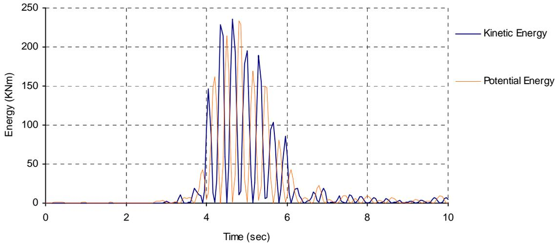
**Figure 7a. Kinetic and Potential Energy for the non-retrofitted structure**
