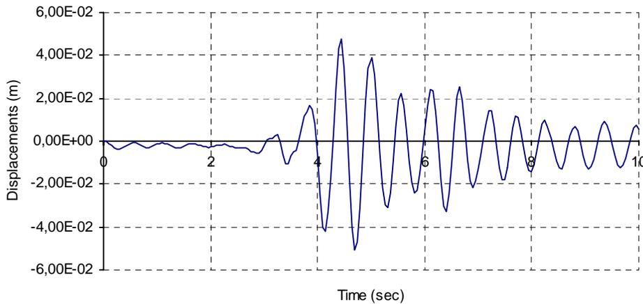
**Figure 8b. Displacement of an indicative joint of the retrofitted structure**
