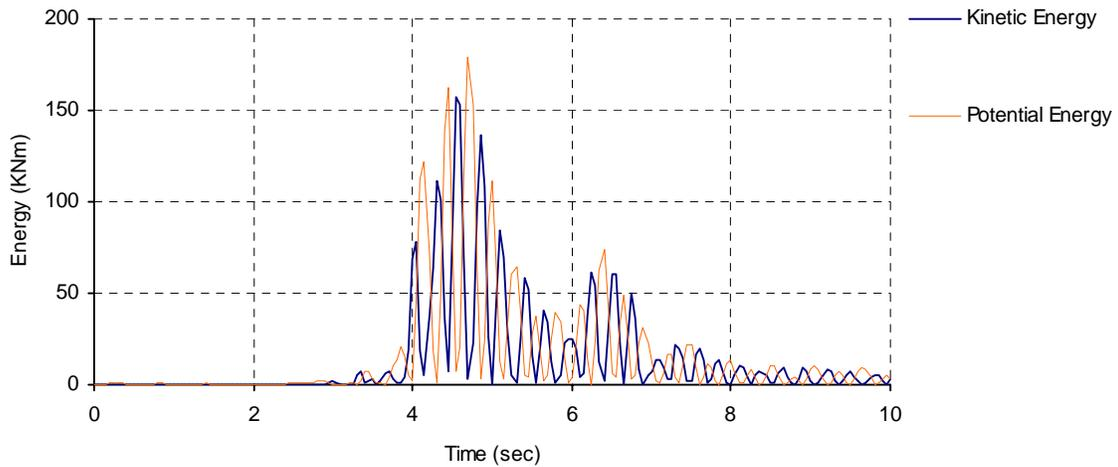
**Figure 7b. Kinetic and Potential Energy for the retrofitted structure**
