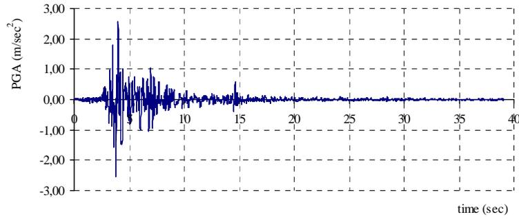
**Figure 5. Athens (1999) earthquake accelerogram**
