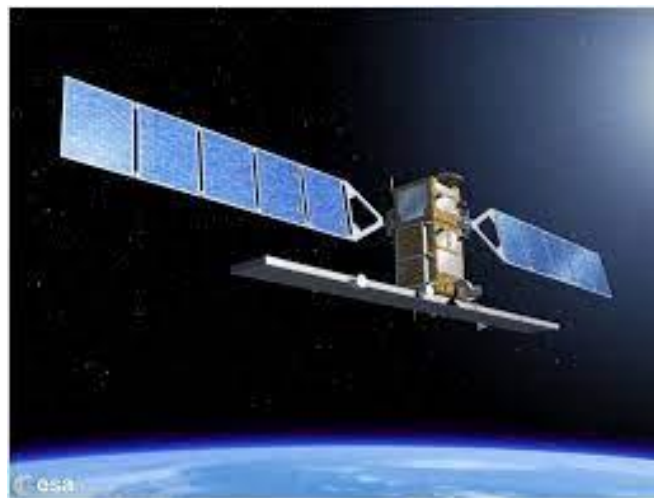
Figure 2: Sentinel 1 satellite with two deployed solar arrays.
