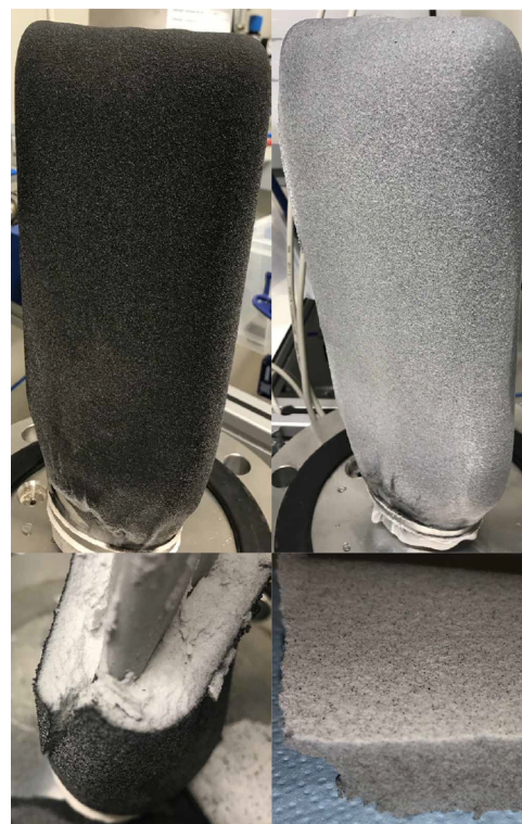
Figure 10. Photographs of the outside and inside of cakes formed by precoat filtration (left) or simultaneous filtration (right) of cellulose fibers and pulverized activated carbon.
