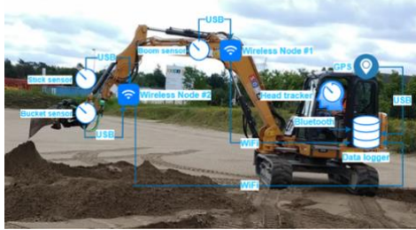
Figure 5. The configuration of the system's hardware on an excavator
