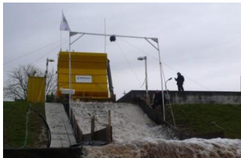
Figure 1.4. Wave overtopping simulator (Bakker, Melis, & Mom, 2013)
