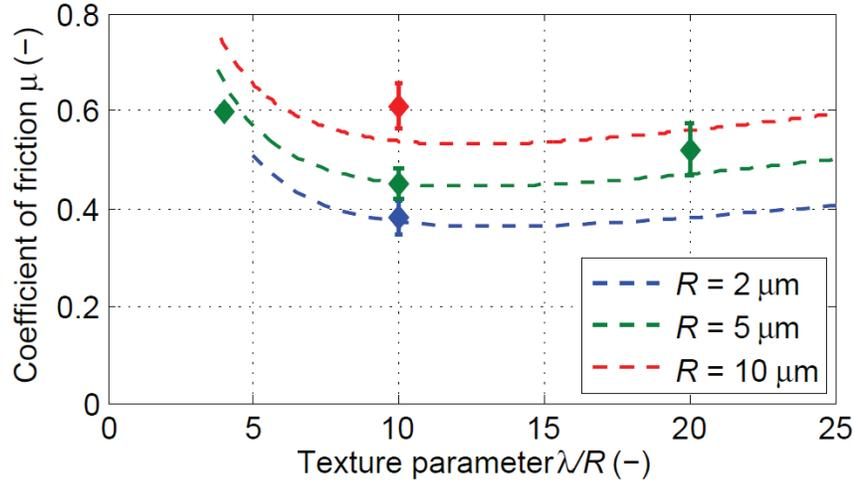
**Figure 6.** Coefficient of friction of the fingerpad sliding against a surface texture as a function of tip radius  $R$  and spacing  $\lambda$ : experimental results (dots) and modeling results (lines).
