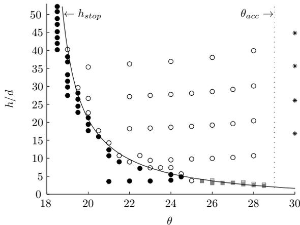
Fig. 2: Overview of DPM simulations for  $\mu^b = 0.5$ , with markers denoting the state: arrested filled-symbols, steady open-symbols, and accelerating \*. The demarcation line is fitted to  $h_{stop}$  in eq. (2) (solid line). Note, circular symbols are for increasing the number of particles and square symbols for decreasing.
