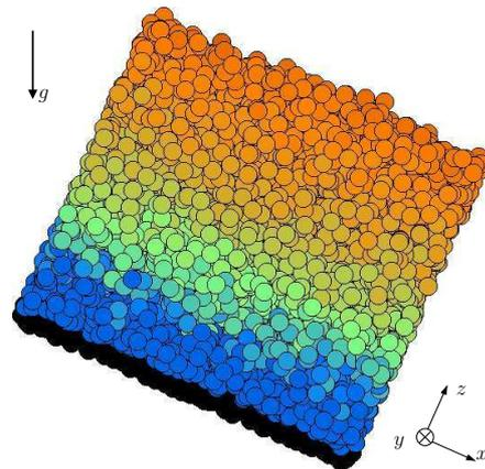
Fig. 1: DPM simulation for  $N = 3500$ , inclination  $\theta = 24^\circ$  and the basal contact friction,  $\mu^b = 0.5$ , at time  $t = 2000$ ; gravity direction  $\mathbf{g}$  as indicated. The domain is periodic in the  $x$ - and  $y$ -directions. In the plane normal to the  $z$ -direction, fixed (black) particles form a rough base while the surface is unconstrained. Colours indicate speed, which increase from slow (blue) at the bottom to faster (orange) towards the free-surface.
