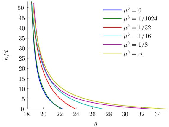
Fig. 3: Demarcation lines  $h_{stop}(\theta; \mu^b)$  between retarding and steady flows for various values of  $\mu^b$ . The demarcation line is fitted to eq. (2).
