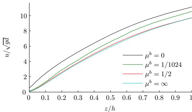
Fig. 6: Flow velocity profile for thick flow with  $N = 6000$  ( $H = 30$ ), inclination  $\theta = 24^\circ$  and bed micro-friction  $\mu^b = 0, 1/1024, 1/2, \infty$ . The flow velocity roughly observes a Bagnold profile, except near the surface and the base. For  $\mu^b = 0$  the flow shows a slip velocity at the base.
