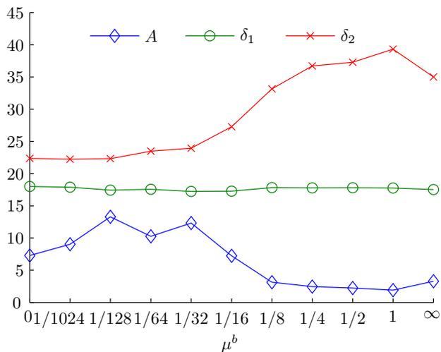
Fig. 4: Figure showing how  $A$ ,  $\delta_1$  and  $\delta_2$  depend on the contact friction coefficient between base and flowing particles,  $\mu^b$ .
