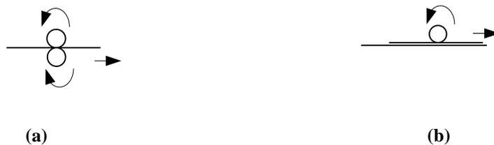
Figure 1-2: A 2d sketch of rollers that move the material. Either a pair of rollers rotates in one direction causing the movement of the paper between them; or, a paper is lying in the feeder and only one roller moves it.
