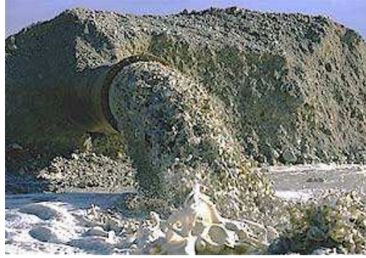
(b) Slurry and sediment transport in pipelines [33].
