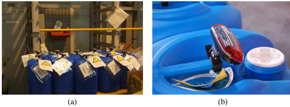
Fig. 1. Application trial in Hull, UK: (a) Chemical containers stored in a warehouse; (b) Detail with a sensor node attached to a container.
