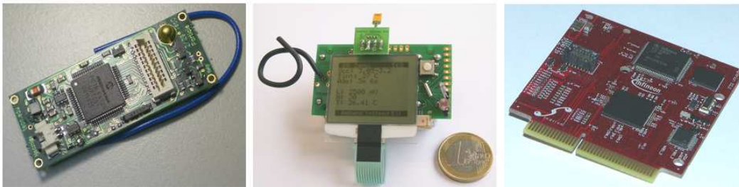
Fig. 2. The three sensor platforms: Particle, \mu Node and Sindrion.
