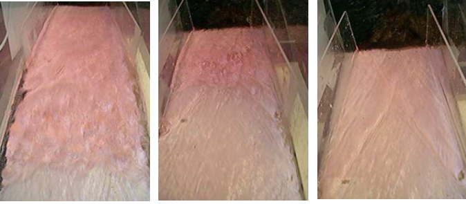
FIG. 4: Multiple states appear for F_0 = 3.07 and B_c = 0.7 , marked by the star in Figure 1. Each transition is induced by blocking or pushing the flow with a small paddle.
