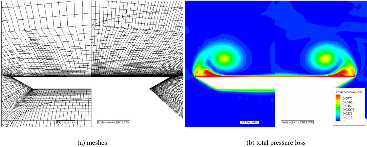
Figure 2: Vortex flow over a delta wing ( $Re=40,000$ ,  $M=0.3$ ,  $\alpha = 12.5^\circ$ ). Comparison of vortex resolution at a cross section of 60% chord between the DG solver Hexadap (left) and the finite volume solver ENFLOW (right). The different meshes are shown on top, and the flow results on the bottom. For the ENFLOW results not the complete cross section is shown.
