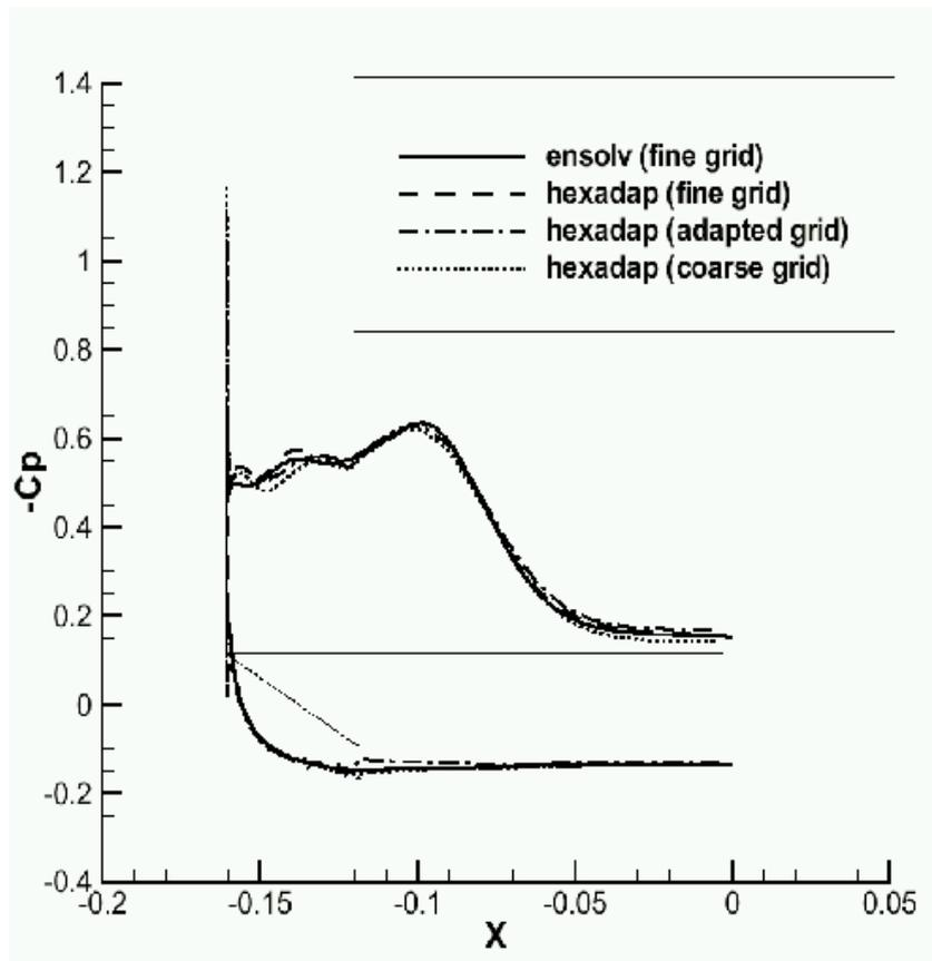
Figure 3: Vortex flow over a delta wing ( $Re=40,000$ ,  $M=0.3$ ,  $\alpha = 12.5^\circ$ ). Comparison of pressure coefficient at a cross section of 60% chord between the DG solver Hexadap and the finite volume solver ENFLOW. For Hexadap results are also shown on the unadapted coarse and fine meshes.
