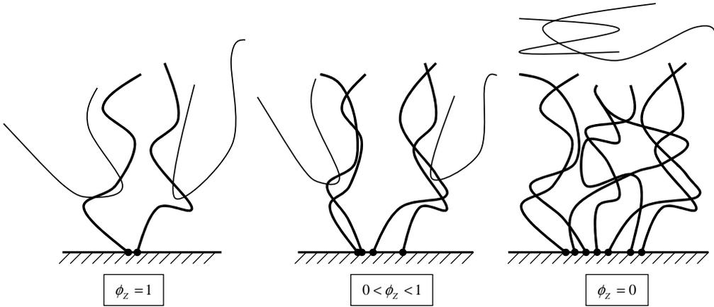
Figure 6: Different grafting regimes. Thick and thin lines stand for the tethered and bulk molecules, respectively
