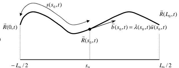
Figure 2: The bond vector of the parameterized chain:  $\lambda(s_0, t)$  and  $\mathbf{u}(s_0, t)$  is the local stretching and the unit tangent vector at point  $s_0$ , respectively.
