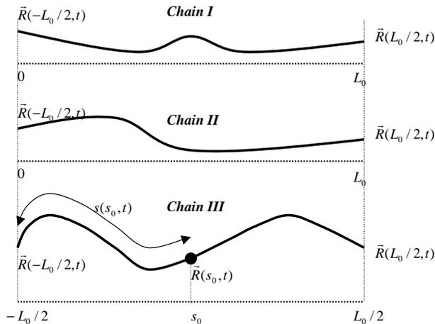
Figure 1: Parameterized curves:  $s$  and  $\mathbf{R}(s_0, t)$  is the physical arclength and the position vector of segment  $s_0$ , respectively;  $L_0$  the equilibrium length of the chain.
