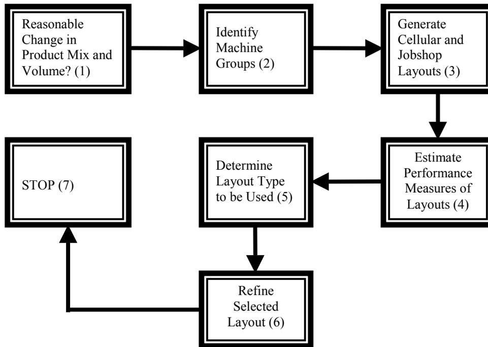
Figure 1. Four phase approach for design and analysis of agile layouts
