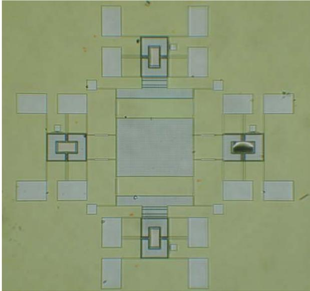
*μSPAM: Two DOF moving plate for probe storage designed by ir. Mihai Patrascu.*
