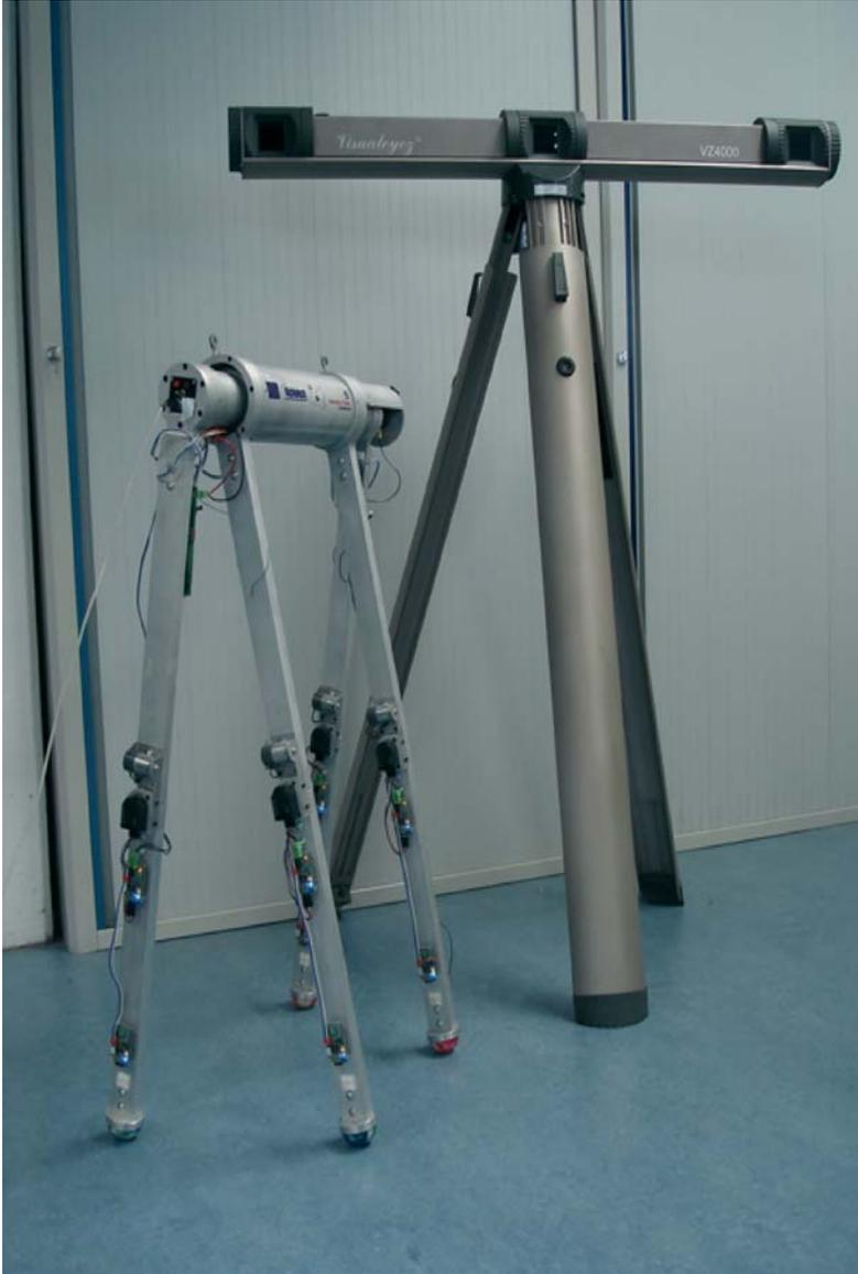
GEOPLEX: *The Robot Dribble* made by ir. Gijs van Oort and ir. Edwin Dertien, and the 3D Tracker.
