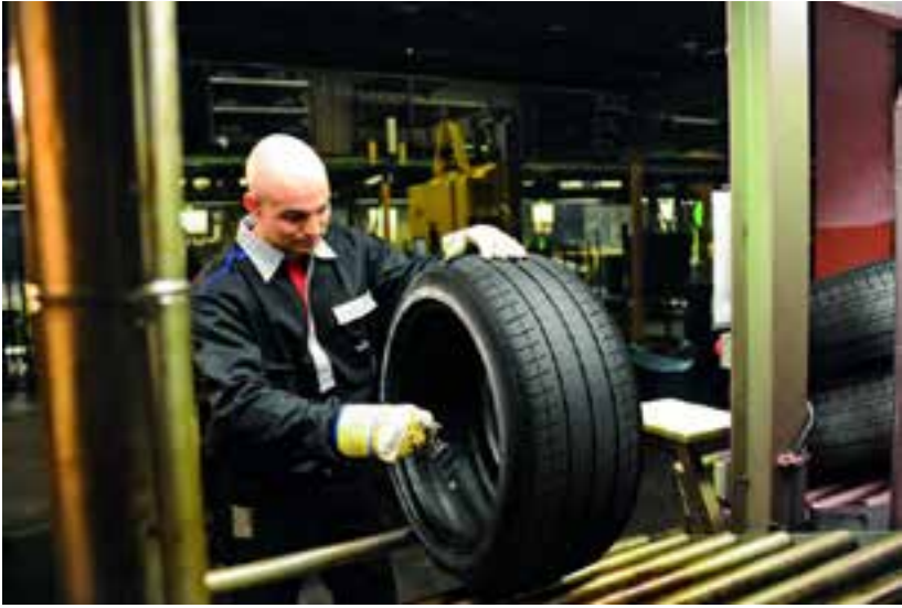
Fig. 21: Apollo's prototype of a tire with natural rubber made from guayule and Russian dandelion [19]
