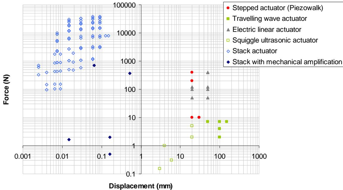
**Figure 1: Force versus displacement chart for the actuators referenced in the detailed review.**
