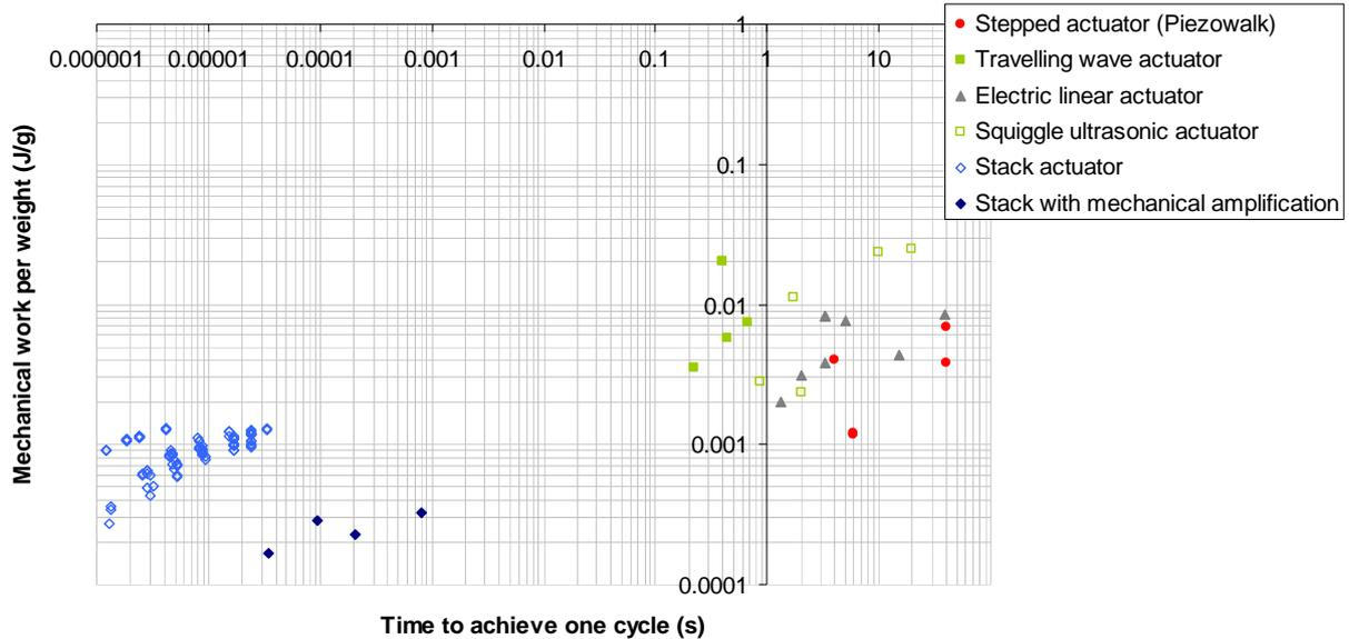
**Figure 2: Time to achieve one cycle versus mechanical work per weight.**
