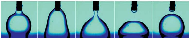
Figure 7. Electrowetting-driven drop oscillations (4).
