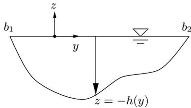
Figure 1: Definition sketch of the geometry.
