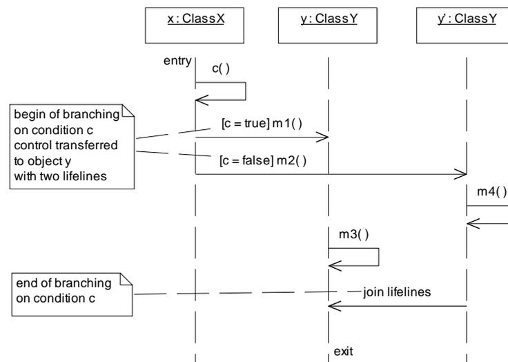
Figure 4. Branching in a sequence diagram to other object with auxiliary lifeline
