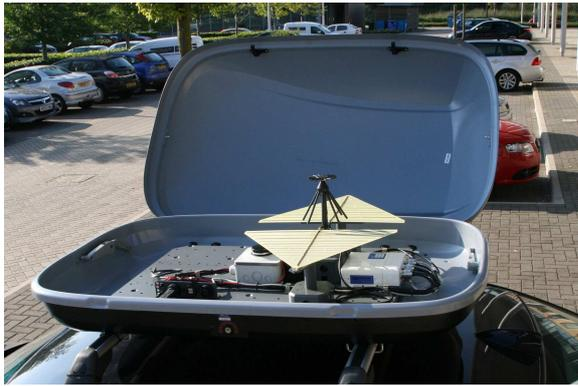
Fig. 2. RFeye system of CRFS
