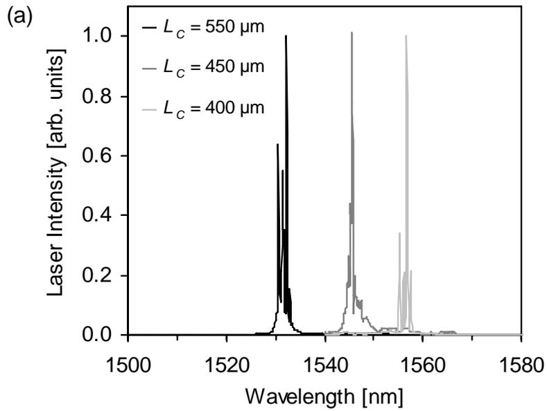
Fig. 8. Laser output spectra for coupler lengths  $L_C$  of 550, 450, and 400  $\mu\text{m}$  (Figure taken from Ref. 23)
