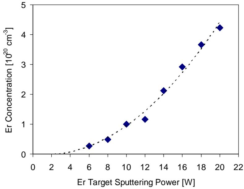
Fig. 1. Er concentration versus Er target sputtering power (Figure taken from Ref. 19)
