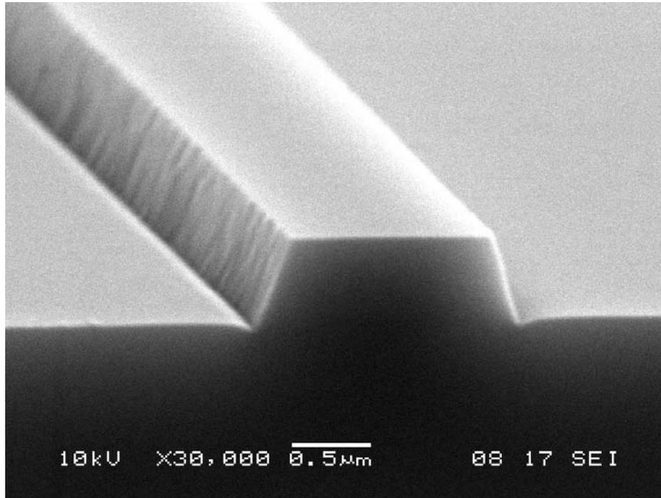
Fig. 3. SEM micrograph profile of a 1.3- $\mu\text{m}$ -wide and 530-nm-deep channel waveguide in  $\text{Al}_2\text{O}_3$  (Figure taken from Ref. 18)
