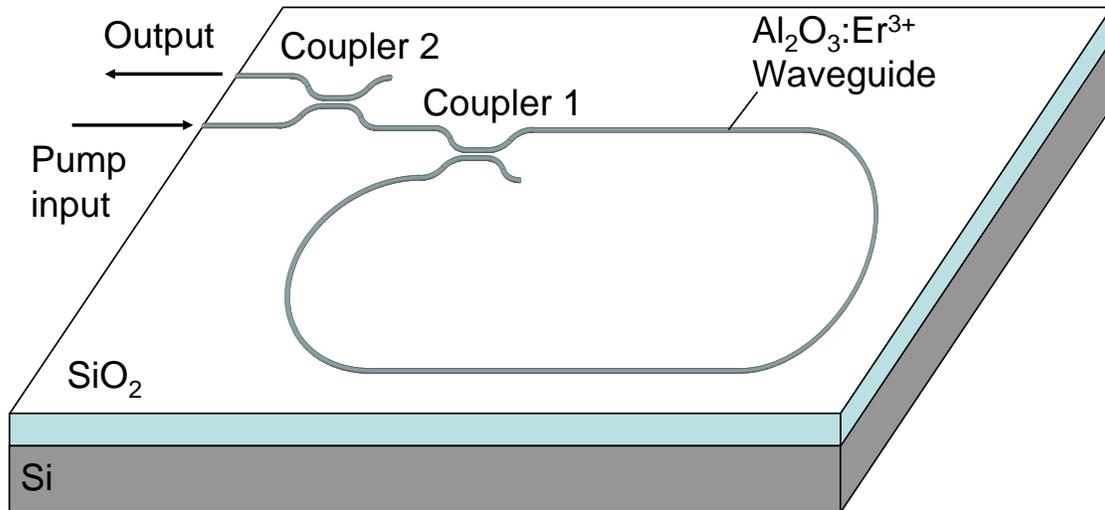
Fig. 6. Schematic of  $\text{Al}_2\text{O}_3:\text{Er}^{3+}$  ring laser (Figure taken from Ref. 22)
