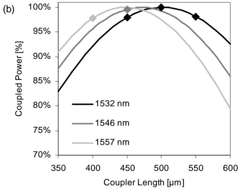
Fig. 9. Simulated coupled power in Coupler 1 vs. coupler length for the observed laser wavelengths and TE polarization. The coupler lengths for which lasing was observed are indicated by the diamonds on the curves. (Figure taken from Ref. 23)
