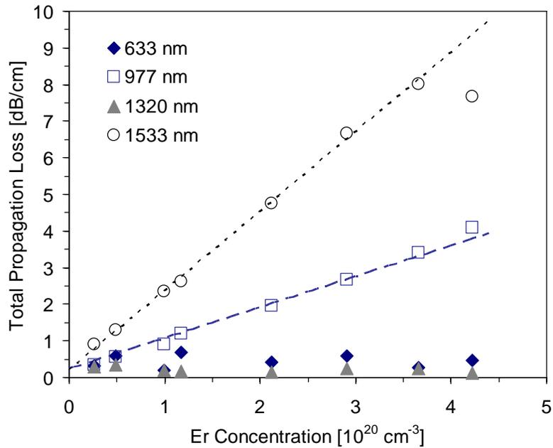
Fig. 2. Total planar waveguide propagation loss at 633 nm, 977 nm, 1320 nm, and 1533 nm as a function of Er concentration. The dashed lines represent the fitted propagation and Er absorption loss at 977 nm and 1533 nm using the average background loss, average confinement factor, and experimentally determined absorption cross sections at each wavelength. (Figure taken from Ref. 19)
