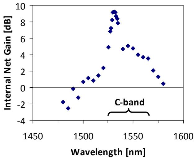
Fig. 5. Internal net gain as a function of wavelength for an amplifier length of 5.4 cm, Er concentration of  $1.17 \times 10^{20}$  cm<sup>-3</sup>, and a launched 977-nm pump power of 80 mW (Figure taken from Ref. 19)
