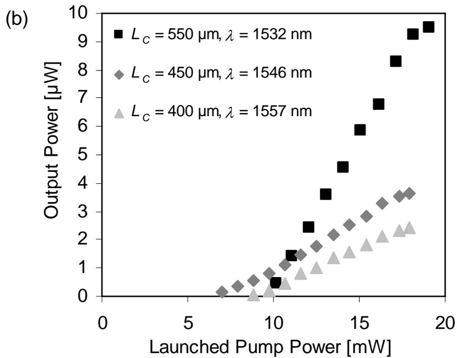
Fig. 7. On-chip integrated laser output power vs. pump power launched into the chip for varying resonator and output coupler length. The resonator length, coupler length, and main lasing wavelength are indicated. (Figure taken from Ref. 23)
