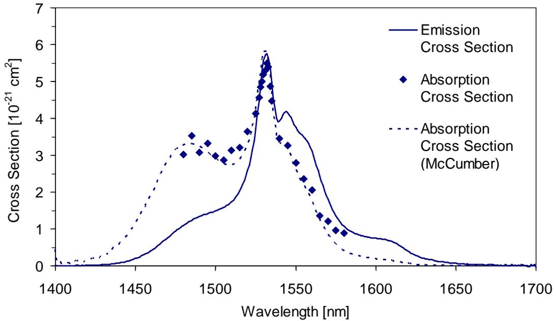
Fig. 4. Emission cross section determined from the luminescence spectra of samples with Er concentrations of 1.00 to  $4.22 \times 10^{20}$  cm<sup>-3</sup>. The absorption spectrum calculated using McCumber theory and measured at single wavelengths in the range 1480-1580 nm are indicated by the dashed line and the plotted points, respectively. (Figure taken from Ref. 19)
