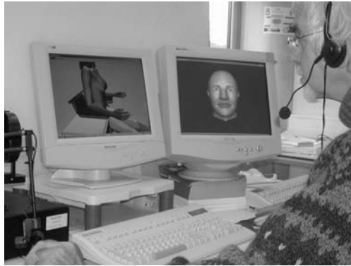
Fig. 1. The INES system. The student is using a haptic device that transforms to an injection needle in the virtual environment (displayed on the left screen ). In this environment the student can interact with a Virtual Patient and perform simple nursing tasks. The performance is monitored by the Virtual Tutor (displayed on the right screen ).
