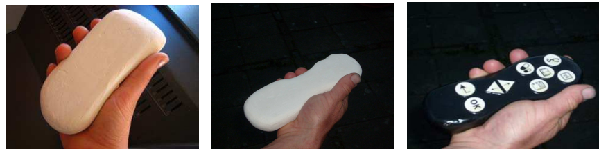
Fig 4. Different stages of the design of remote control.
