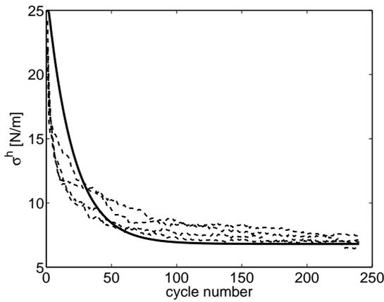
**FIGURE 3.** Evolution of the pressure at the start of a each cycle ( $\gamma = 0$ ). Dashed curves show result for 4 different simulations, the solid curve shows results of the improved model.
