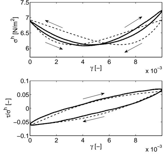
FIGURE 2. Evolution of pressure, and the shear stress over pressure ratio during a cycle after 200 cycles. Arrows indicate the direction of shear; for a more clear picture averages are taken over the last 50 cycles. Solid curves are averages of the simulation results and the dashed curves lines are a fit using the model (both the improved as the original model show the same behaviour)
