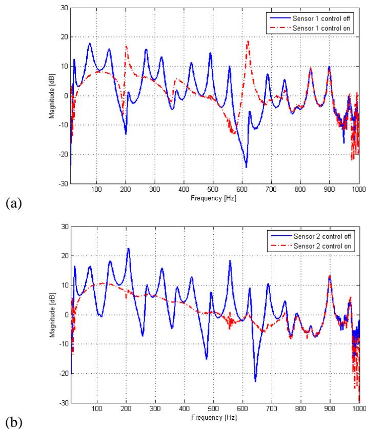
Figure 8. Total pressure response: with real-time feedforward configuration 2 control. (a) sensor position 1; (b) sensor position 2.
