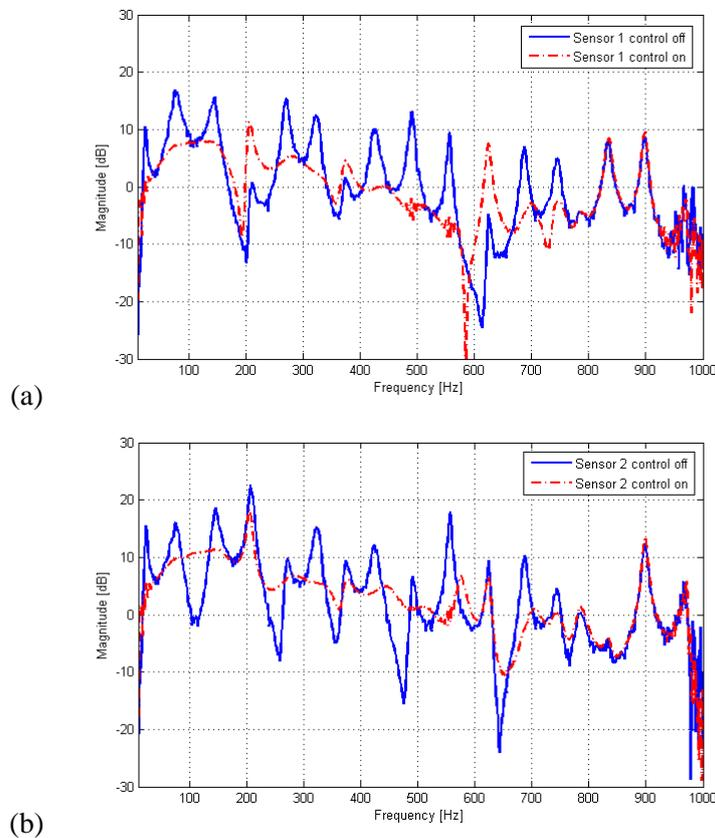
**Figure 6.** Total pressure response: with real-time feedforward configuration 1 control.
