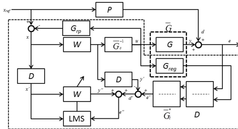
Figure 3. Regularized modified filtered-error adaptive control scheme with IMC.
