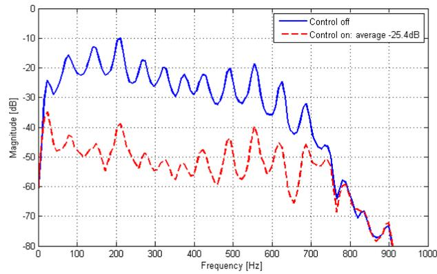
Figure 7. Reflecting pressure response: with real-time feedforward configuration 2 control.
