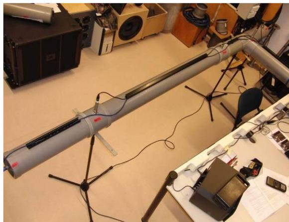
Figure 2. Experiment set-up for real-time control.
