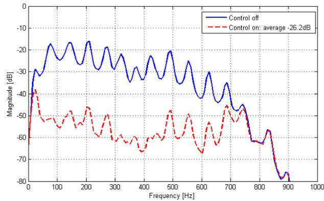
**Figure 5.** Reflecting pressure response: with real-time feedforward configuration 1 control.
