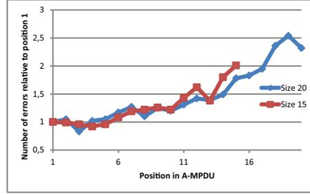
**Fig. 9.** The number of errors relative to the number of errors on the first place plotted against the location of an MPDU in an A-MPDU
