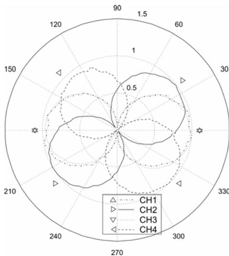
**Figure 7. Sensitivity pattern of the sensors at 1.7kHz, rotated around the  $z$ -axis. Triangles show the measured sensitivity directions. Theoretically for sensors in free space, all channels should yield a 45 degrees angle with the  $x$ - or  $y$ -axis.**
