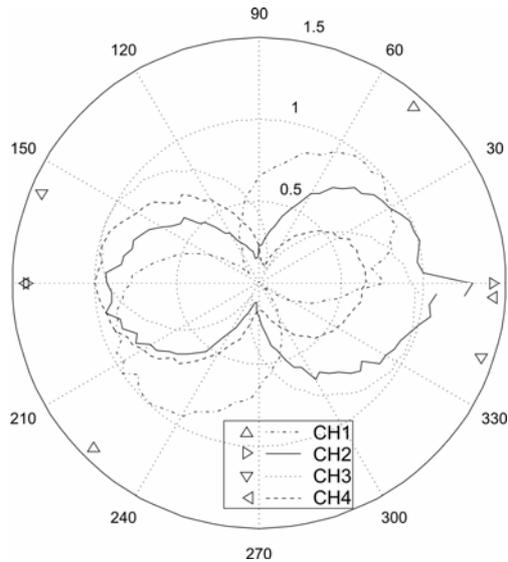
**Figure 6. Sensitivity pattern of the sensors at 1.7kHz, rotated around the  $x$ -axis. Triangles show the measured sensitivity directions. Ideally, signals of channel 2 and 4 have directions of 0 and 180 degrees, channel 1 at 45 and 225, channel 3 at 135 and 315 degrees.**
