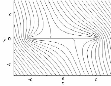
Figure 4. Streamlines of the flow around a plate of width  $2c$ , where the velocity at infinity makes an angle  $\alpha = \pi/3$  with the  $x$ -axis. The streamlines are lines of constant  $\psi$  with  $\psi$  from Eq.(16.).
