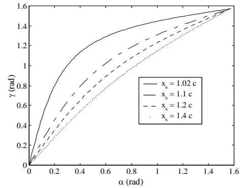
Figure 5. The angle  $\gamma$  of the velocity at the sensor location  $(x_s, 0)$ , as a function of the angle  $\alpha$  of the incoming wave, with  $x_s$  as a parameter.
