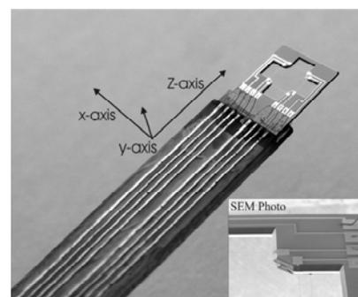
**Figure 1.** The integrated three-dimensional particle velocity sensor, composed of four pairs of sensor wires.
