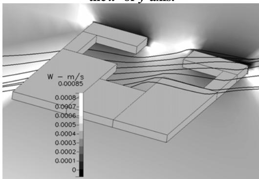
**Figure 8. Visualization of results from computational fluid dynamic calculations. Streamlines are 'bent' around the edges of the probe surface.**
