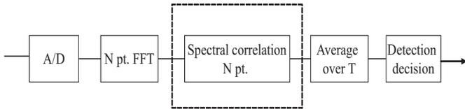
Fig. 2. System level architecture of spectrum sensing with the cyclostationary feature detection option
