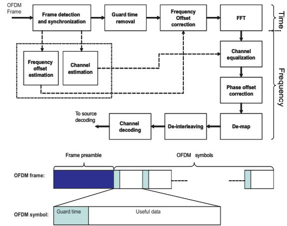
Fig. 4. Basic OFDM processing tasks
