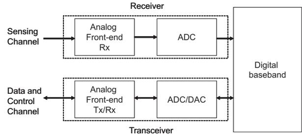
Fig. 1. The physical layer architecture of a Cognitive Radio node
