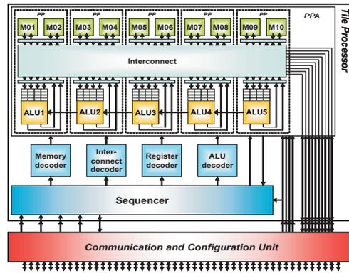
Fig. 6. An example of DSRH: a Montium processor
