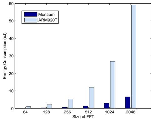
Fig. 7. Energy consumption (in  $\mu\text{J}$ ) comparison between the Montium and ARM
