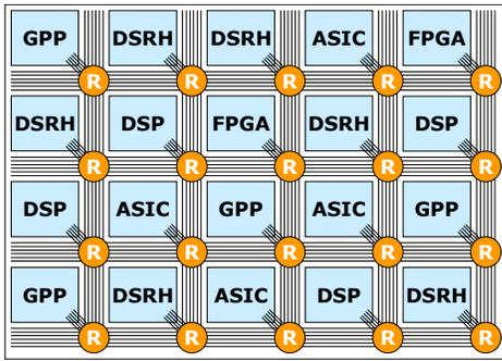
Fig. 5. An example of a heterogeneous System on Chip (SoC). DSRH = Domain Specific Reconfigurable Hardware
