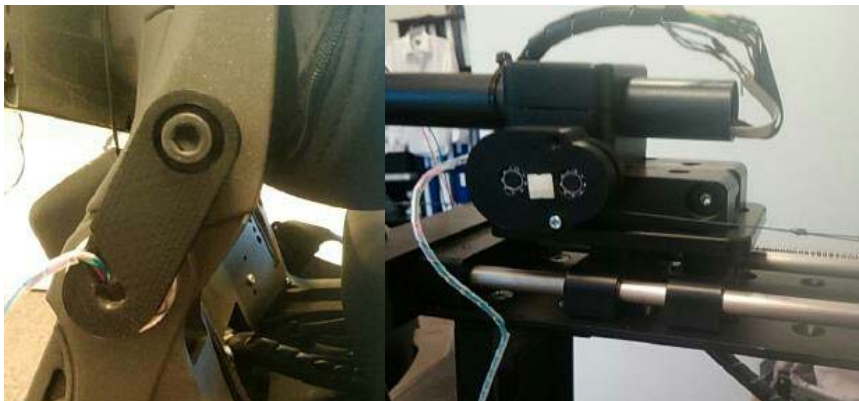
Figure 6: Picture of wheelchair back seat absolute encoder measuring the angle of the back seat to the seat cushion (left). Picture of joint position absolute encoder (DOF3) measuring forward-backward translation (right).
