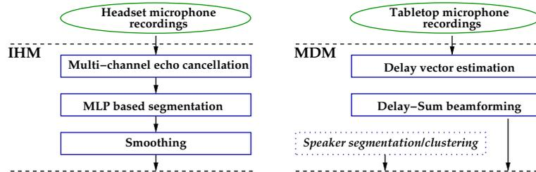
Fig. 2. Front-end processing of IHM and MDM data.
