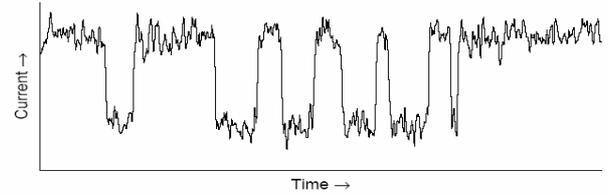
**Figure 5: Time domain measurement of the drain current: discrete constant amplitude current steps occur, known as a "Random Telegraph Signal" (RTS)**
