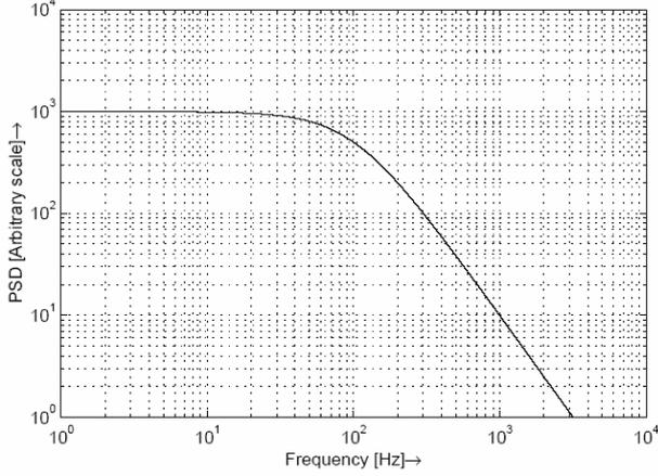
**Figure 9: PSD of a Random Telegraph Signal (RTS)**
