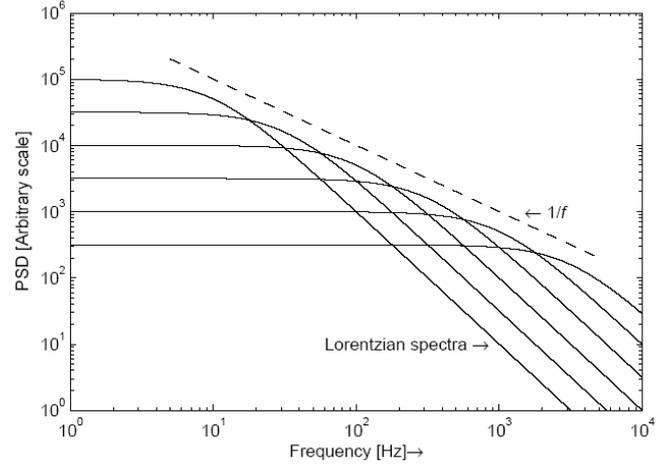
**Figure 11: Adding several Lorentzian spectra can result in a spectrum that closely resembles 1/f noise**
