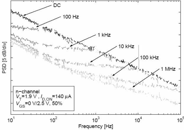
**Figure 3: Effect of switching frequency on noise reduction: all lines converge at low frequency so the switching frequency is irrelevant for the LF noise reduction.**
