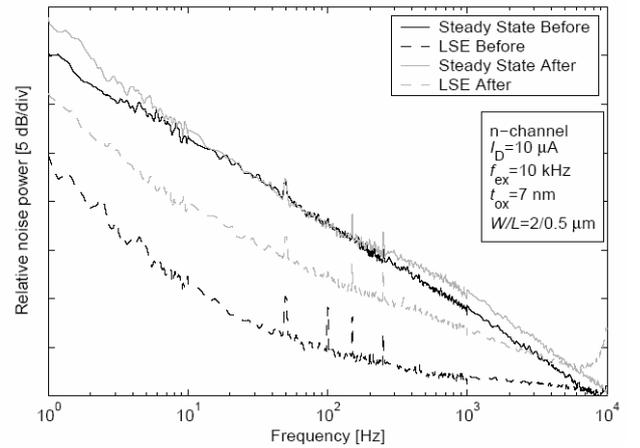
**Figure 16:** Effect of hot electron damage on the constant and switched bias noise spectrum: before damage the noise reduction is well above 6dB. After damaging the device there is just 6dB (as expected from signal theory)
