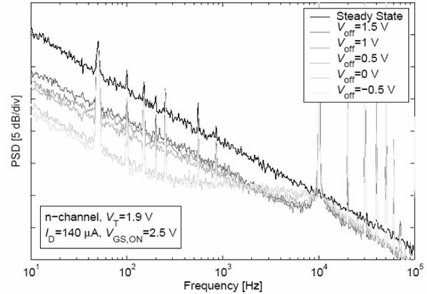
**Figure 2: LF noise spectrum for various off-voltages. Whereas 6dB is expected, more noise reduction is found if the off-voltage is lowered below the threshold ( $V_{TH}=1.5$  Volt in these old devices)**
