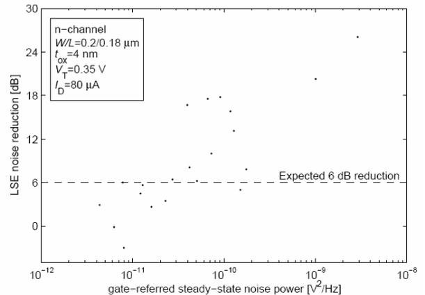
**Figure 6: Noise reduction found under LSE versus the noise for steady state biasing: large reductions up to >20dB are found, but also sometimes increased noise (below 6dB line)**
