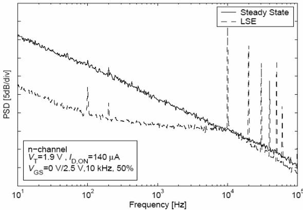
**Figure 1: Power Spectral Density of the noise of HEF4007 devices at constant bias (top line) and Large Signal Excitation (LSE) at 10kHz (low line): below the switching frequency noise reduction is observed.**
