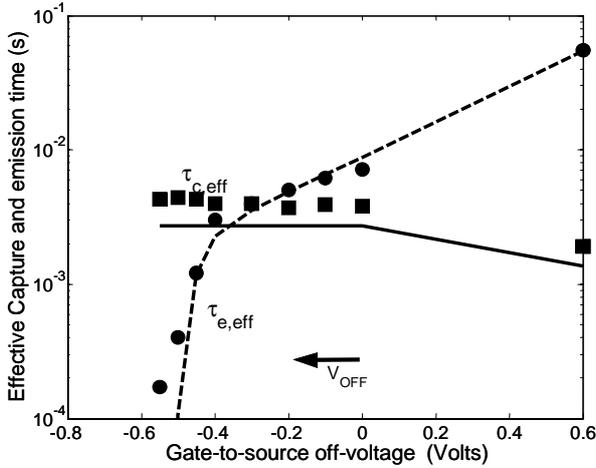
**Figure 15:** Measured and predicted effective cyclo-stationary capture and emission times versus gate-source off-voltage ( $V_{GSon} = 0.6V$ ,  $V_{DS} = 50$  mV, duty-cycle = 50%).
