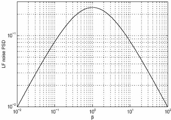
**Figure 10: PSD "plateau" at low frequency of an RTS signal as a function of  $\beta$  : if the ratio is 1 ( $\tau_e = \tau_c$ ), power is maximized**
