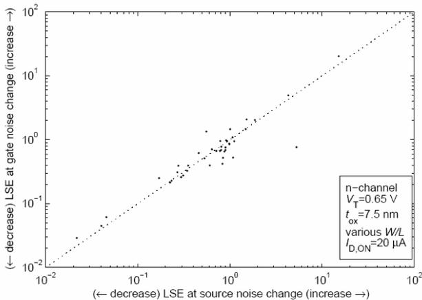
Figure 8: Noise reduction found for gate switching and for source switching. Their effect is strongly correlated, i.e. source switching has almost the same effect.
