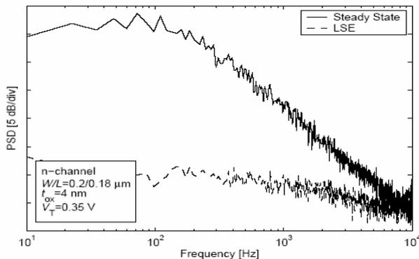
**Figure 4: PSD of the drain current for a device dominated by RTS noise: a flat LF part and -20dB/decade HF roll-off are found. For LSE the noise is strongly reduced.**
