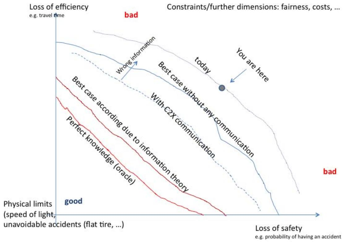
Figure 1: The design space of inter-vehicle communication.
