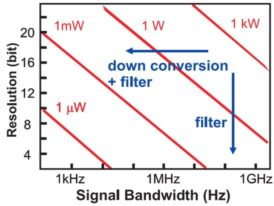
Figure 2: Power consumptions of ADC's as a function of signal bandwidth and resolution
