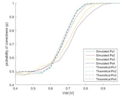
Fig. 4. Simulated and theoretical E-p curves for sum outputs
