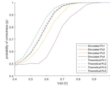
Fig. 3. Simulated and theoretical E-p curves for carry outputs
