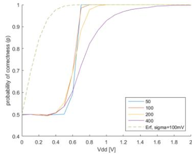
Fig. 1. CMOS inverter simulations for various noise scales.
