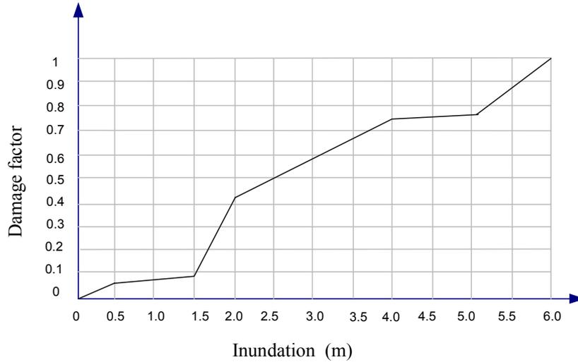
Figure 5 Example of a damage function for households
