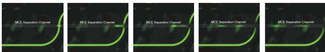
Figure 2 - Formation, propagation, diffusion-induced broadening, and MCE separation of a 30 picoliter plug of Fluorescein and Rhodamine-6G through a gel-matrix in a microfluidic channel
