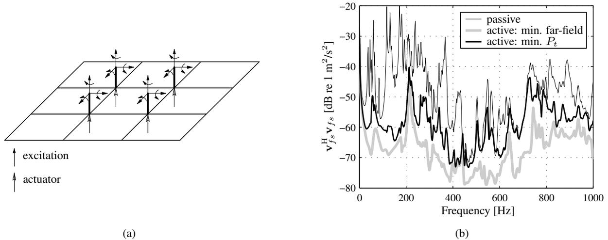
Figure 4: Far-field sensor response with minimization of transmitted power.
