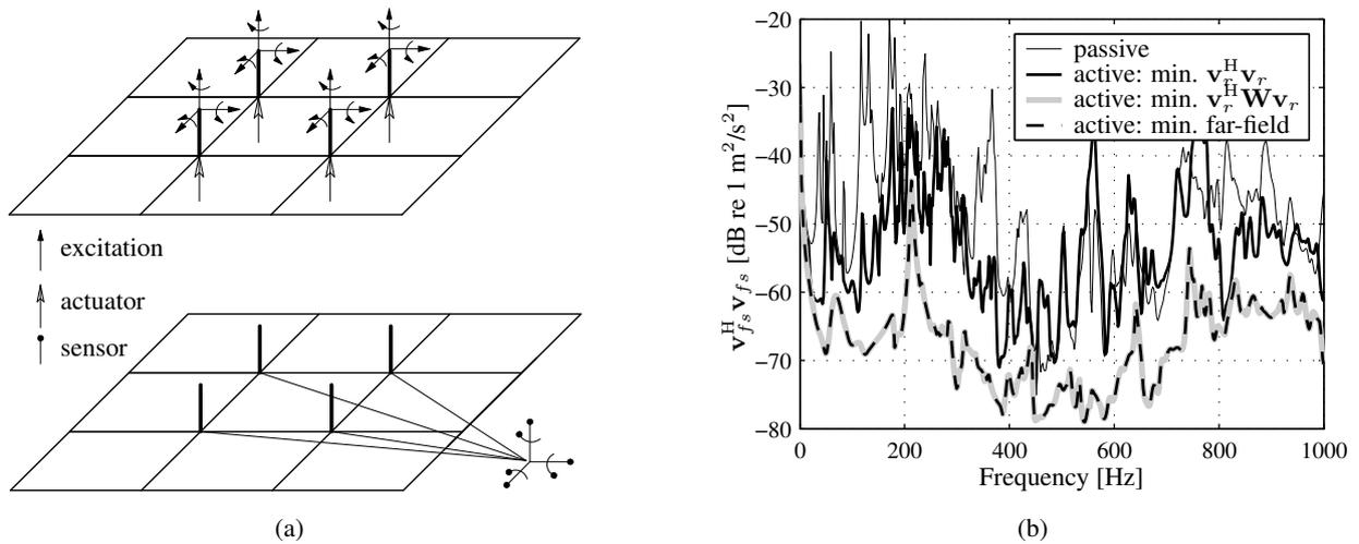
Figure 5: Far-field sensor response for minimization of the velocities at the mount positions of the receiver (near-source sensor set 1).
