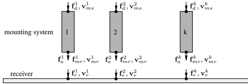
Figure 2: General model of a hybrid isolation system.
