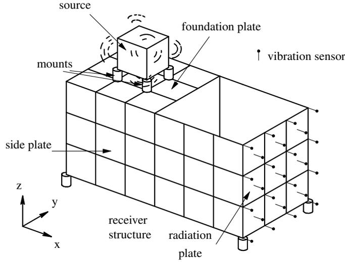
Figure 3: Sketch of the hybrid isolation model with far-field sensor set at TNO TPD.
