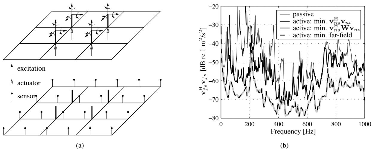
Figure 6: Far-field sensor response for (weighted) minimization of a velocity sensor set at the foundation plate (near-source sensor set 2).
