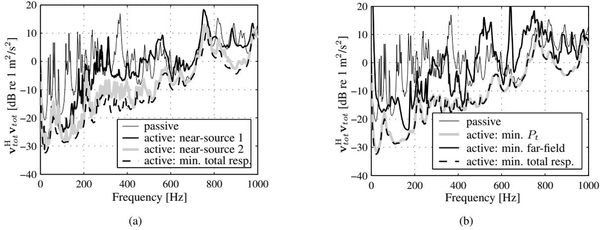
Figure 7: Influence of different cost functions on the total response of the receiver structure.
