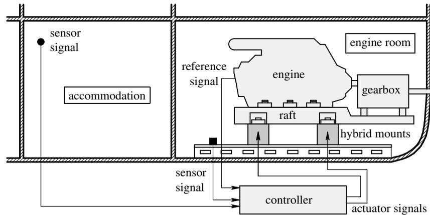
Figure 1: A schematic overview of a hybrid isolation system for a ship engine.
