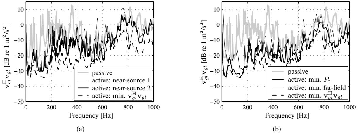
Figure 8: Influence of different cost functions on the global far field response (the side and radiation plate of the receiver structure).
