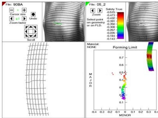
Figure 14: FLD measurement Nakazima sample around plane strain
