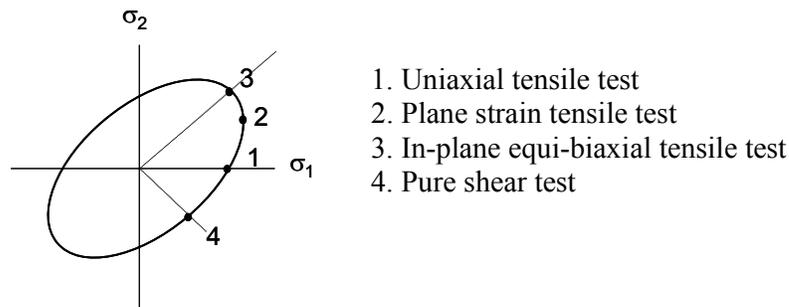
Figure 1: Four basic mechanical tests
