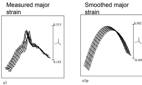
Figure 15: Major strain distribution before and after smoothing
