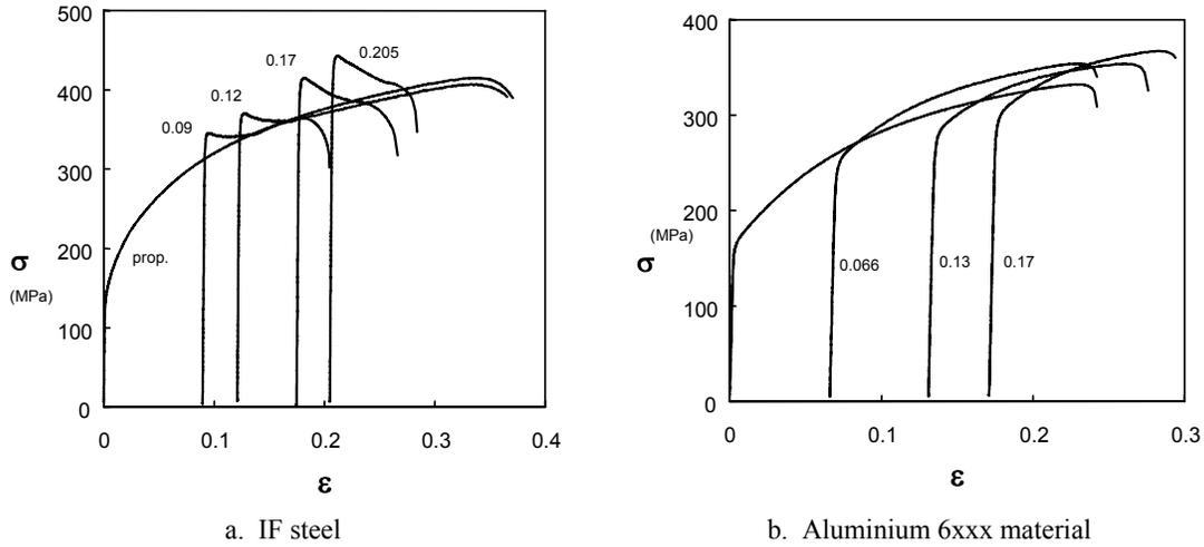
Figure 11: Tensile test curves after various equi-biaxial prestraining; numbers indicate the thickness strain of the pre-deformation.
