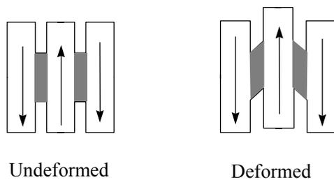
Figure 9: Geometry of the pure shear test specimen
