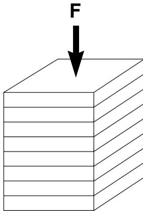
Figure 7: Stacked sheet specimen for the compression test
